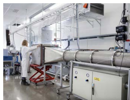
In Camfil's molecular media test rig in Trosa, Sweden, various filtration technologies are challenged with different gases at realistic concentrations against a wide range of temperature, humidity, and airflows.
